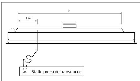
This requires a thin tube to insert through the nozzle into the plenum. Please note that extravent units use an open nozzle to perform the measurement. Inserting the measuring tube into a closed hole can damage the seal of the extravent strip and cause noise problems.
